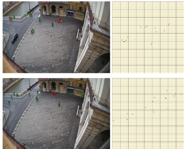
Fig. 3: Examples of the output of our social distance measurer module. Left: images with the detected pedestrians. Right: 2D projection on a virtual planar surface obtained through homography. Green color means a safe placement; red color indicates violations of the social distance rule. Image Courtesy of [11].
