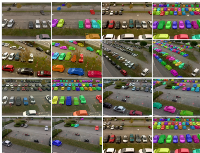
Fig. 1: Examples of the output of our vehicle counting solution. We show input images captured by smart cameras and the detected vehicles by our CNN-based technique.
