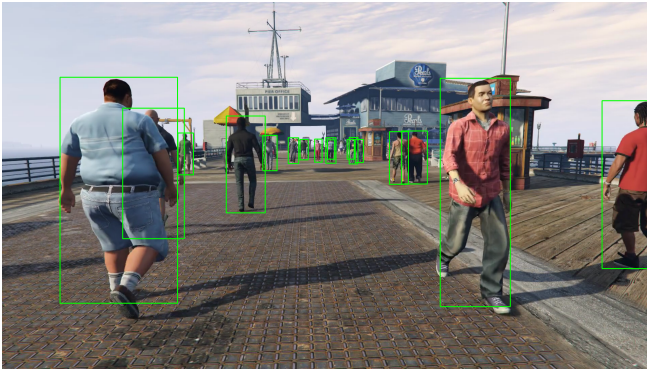
Fig. 2: Sample of our ViPeD dataset. Images and bounding boxes localizing the pedestrians are automatically gathered from a virtual-world. Image Courtesy of [7].
