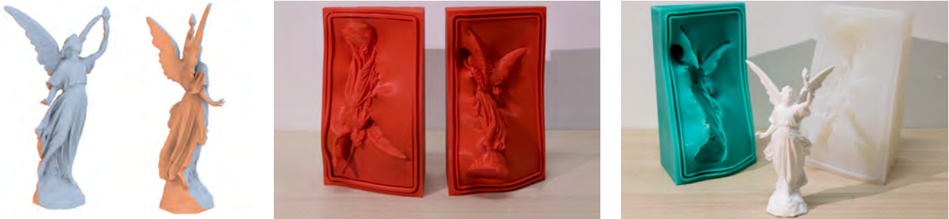
Fig. 1. Our approach automatically generates the shape of silicone molds for casting an input 3D mesh. After computing a segmentation of an input mesh into moldable pieces (left), we design and 3D print a set of metamolds (middle, in red). The actual mold pieces (right, in green and whitish) are produced by pouring liquid silicone onto the metamolds, then assembled and used to cast copies of the input model.
