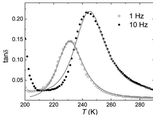
Fig. 5. Thermally activated peak in supercooled PYR<sub>14</sub>-TFSI. The continuous line is a fit according to Eq. (1)
