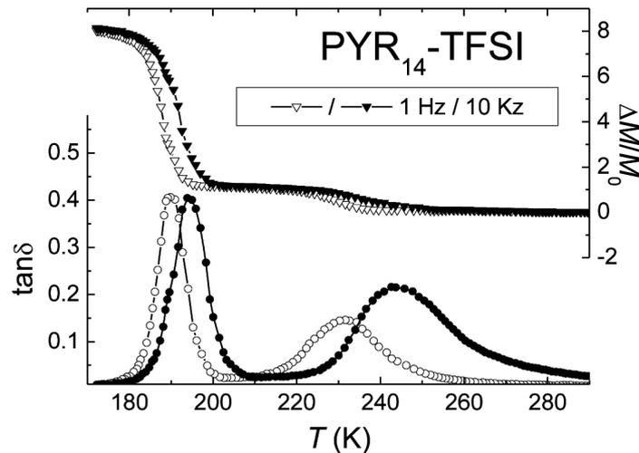
Fig. 4. DMA spectra of the pocket containing PYR<sub>14</sub>-TFSI, measured at two frequencies
