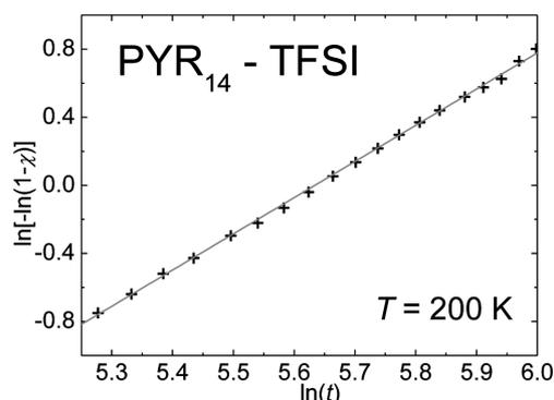
Fig. 7. Isothermal Avrami plot for the cold crystallization process, obtained from an isothermal DMA measurement at  $T = 200$  K
