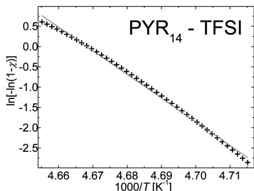
Fig. 8. Non-isothermal Avrami plot for the cold crystallization process. The continuous line shows the best linear fit curve
