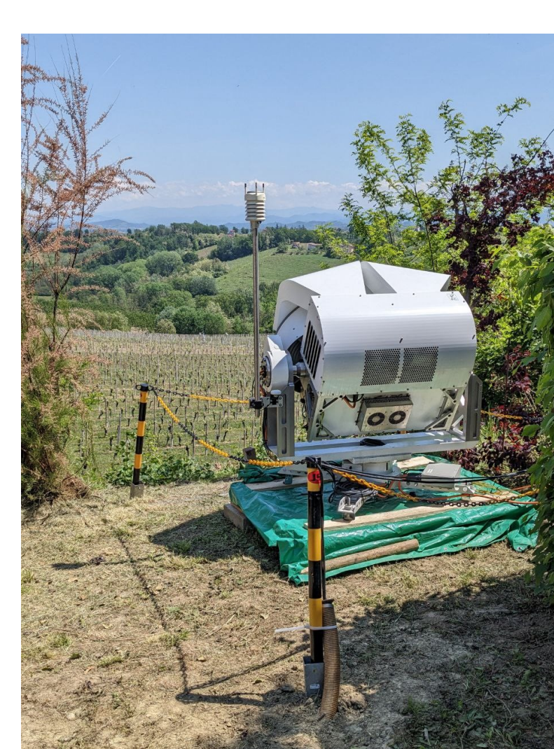
Fig. 5. The polarimetric W-band cloud radar at the Tenuta Cannona site. The radar is located about 100 m from the plots. The radar is pointed to 30° elevation.
