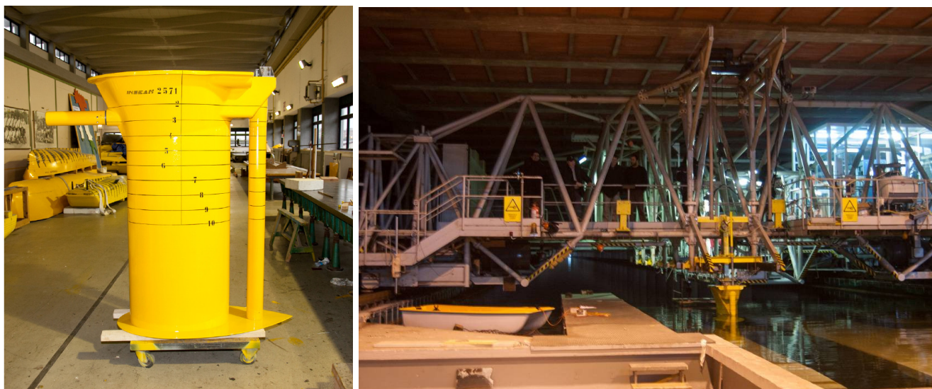
Figure 1: Left: Snorkel mast model. Right: INSEAN Tank n°1. The snorkel mast is mounted below the carriage through a designed support which rigidly fixes the mast at a given immersion.
