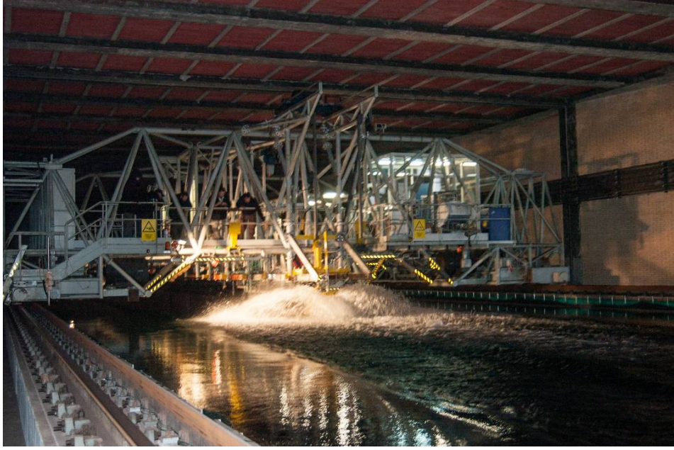
Figure 2: INSEAN Tank n^{\circ}1 . Rear view of the violent flow generated by the snorkel mast moving at 6m/s .
