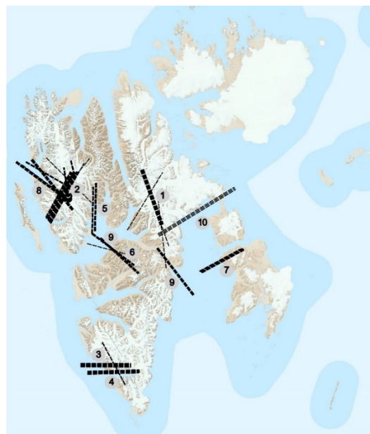
Figure 5. All flight lines covering an area of approximately 700 sq. km in the period 09 June 2020–20 September 2020. Ground resolution varies between 10–30 cm for the RGB images and 20–50 cm for the hyperspectral data.
