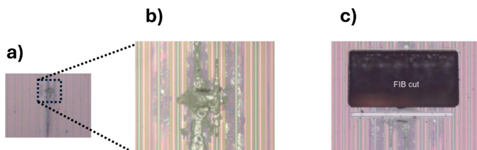
Fig. 1. Optical images of the sample at 10\times (a), 50\times of magnification before (b) and after (c) FIB cross-sectioning.
