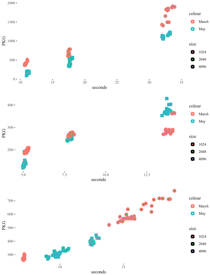
Fig. 1. Comparison between different versions of the VMs on the OneMax problem; from top to bottom: node, bun, deno
