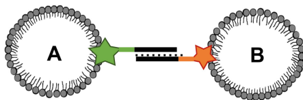
Fig. 2. Sketch of a pair of oil-filled droplets in water, to which complementary strands of ssDNA oligonucleotides are attached: The surfaces of the droplets are composed by single-tail surfactant molecules like lipids with a hydrophilic head on the outside and a hydrophobic tail on the inside, thus forming a boundary for the oil-in-water droplet. By adding some single-strand DNA to the surface of a droplet, it can be ensured that only desired connections to specific other droplets with just the complementary single-strand DNA can be formed. Please note that the connection of the droplets in this picture is overenlarged in relation to the size of the droplets. In reality, the droplets have a radius of 1–50 \mu\text{m} , whereas a base pair of a nucleic acid is roughly 0.34 nm in length [1], such that the sticks of connecting DNA strands are roughly 5 nm long.
