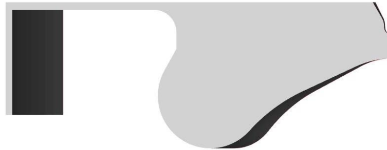
Figure 1. Cross section of a 60° sector of the combustion chamber, corresponding to one injector hole.
