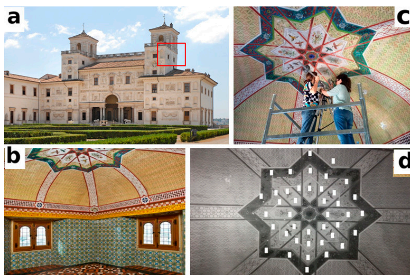
Figure 7. (a) Villa Medici; (b) the Turkish room; (c) NMR probe mounted on its metal arm while measuring the vault surface; (d) Matrix of area analyzed on the vault by NMR.
