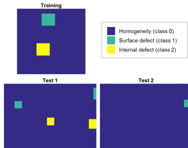
Fig. 8. Ground truth corresponding to the three regions considered for training classifiers and test predictions.
