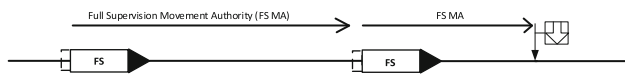
Fig. 1 Overview of full moving block system type without trackside train detection taken from [75]
