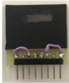
Figure 6: a picture of the interdigital circuit with GNPs and MoS2 on the top.
