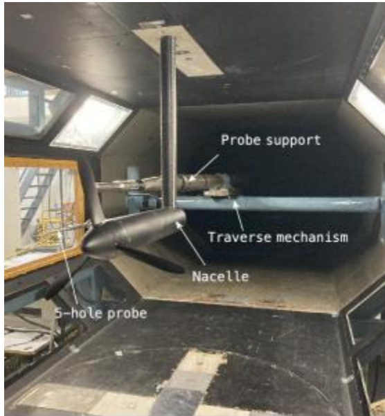
Figure 1: Propeller setup in the Low Turbulence Tunnel
