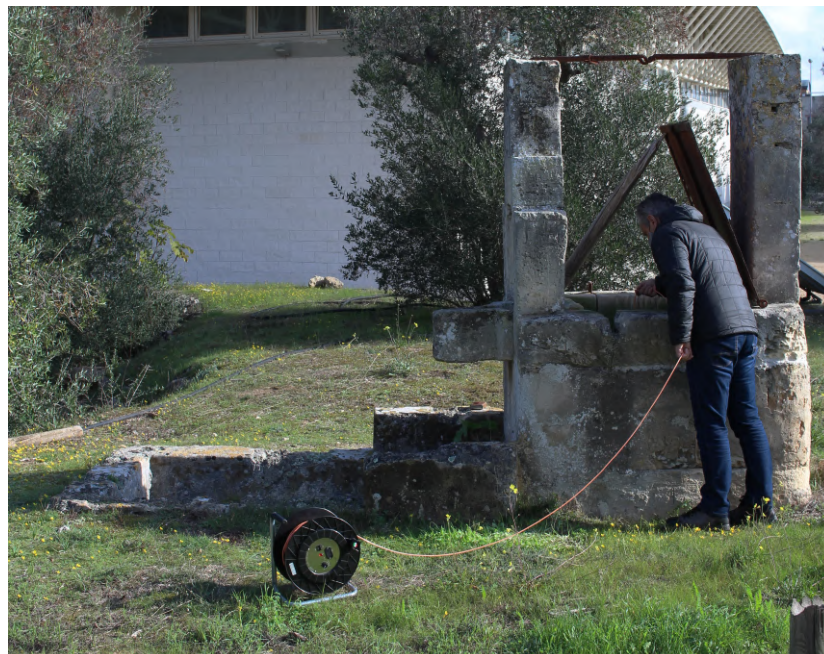
Figure A4. The descent of the electronic meter in the Benessere Well. Photo by Luca Ciricugno.
