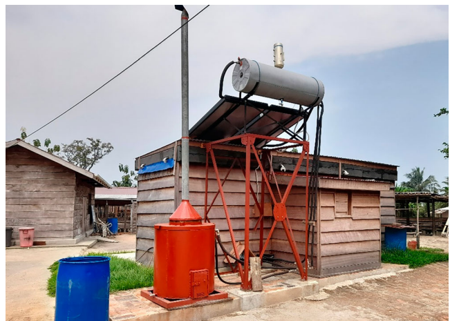
Figure 3. Back side of the completed kiln with the small technical room (hosting the control and the electric panel), the furnace, the flat solar thermic collector and the water tank. Note: The seasoning area of the sawmill can be seen beyond the kiln.
