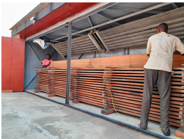
Figure 12. View of the inner part of the kiln with the stack at the end of the drying process.
