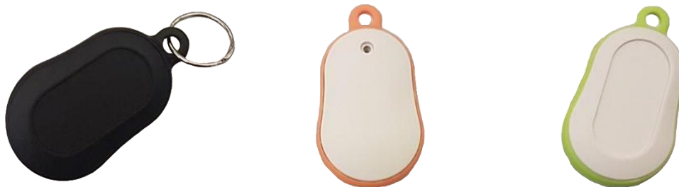
Figure 5 BLE beacons used as environmental sensors and for detecting social interactions. On the top: the GlobITag testing platform; on the bottom: the custom NESTORE beacon developed by Flex.
