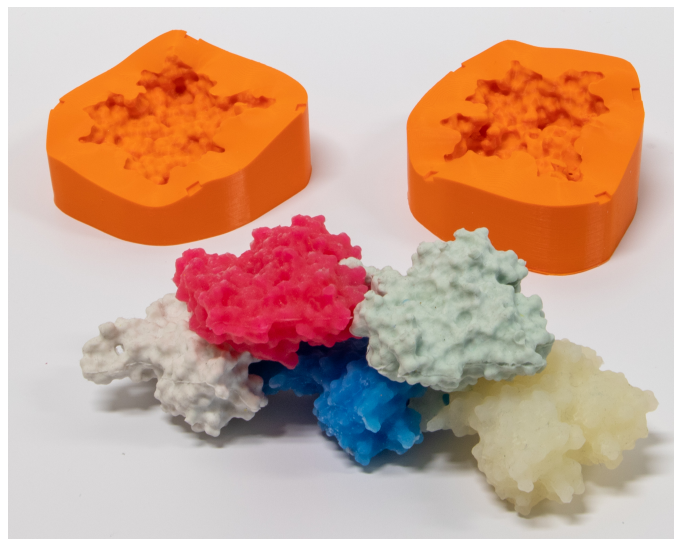
Fig. 9. The rigid 3D printed mold for the F-actin monomer and a fragment of filament assembled using five identical subunits cast from the same mold. To better appreciate the helical structure of the filament see Figure 1.f.
