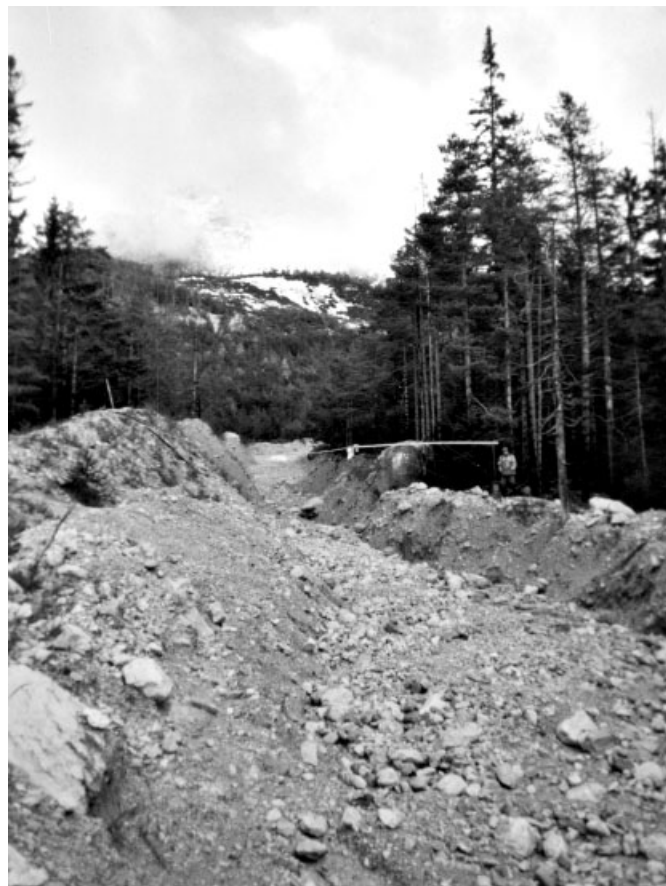
Figure 4. Downstream view of station 3; steel rotating arm with hanging ultrasonic sensor and videocamera in foreground
