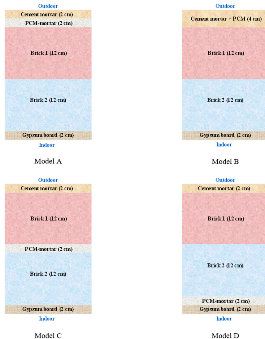
Figure 16. Schematic representation of the PCM location in the wall structure.
