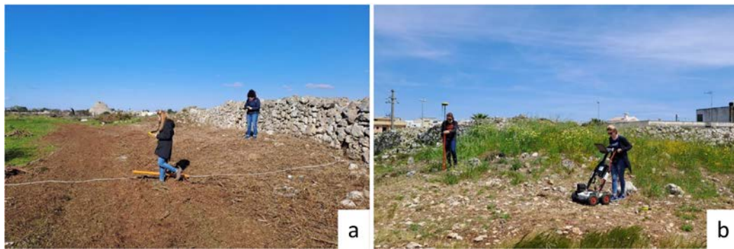
Figure 2. Geophysical instruments used for the acquisition of data: (a) electromagnetometer mini-explorer (GF instrument); (b) GPR with multifrequency antenna 200/600 MHz (IDS).
