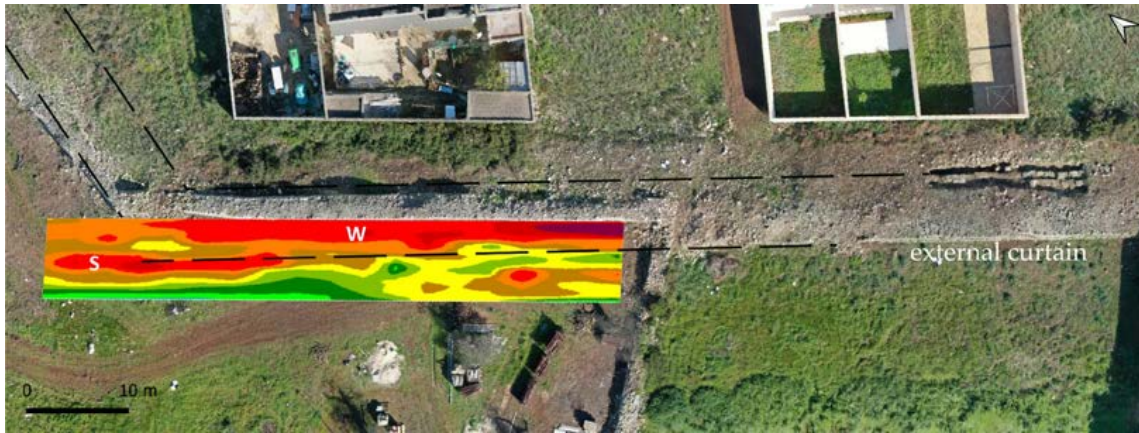
Figure 6. Area 1: georeferenced depth slice (depth of 0.87–1.25 m) over the drone orthophoto, with indication of the anomaly referable to the buried Messapian city walls (named W) and other anomalies probably referable to structures related to the buried walls (named S). The elongated high resistivity anomaly, designated by colors from red to purple (W) and indicated by the black dashed line, aligns with a section of visible city walls (external curtain) in the adjacent area.
