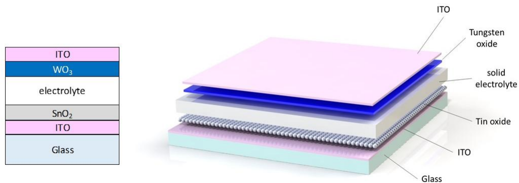
Figure 1 – Cross-sectional view of the device (left side) and axonometric diagram (right side) reporting all the layers deposited.
