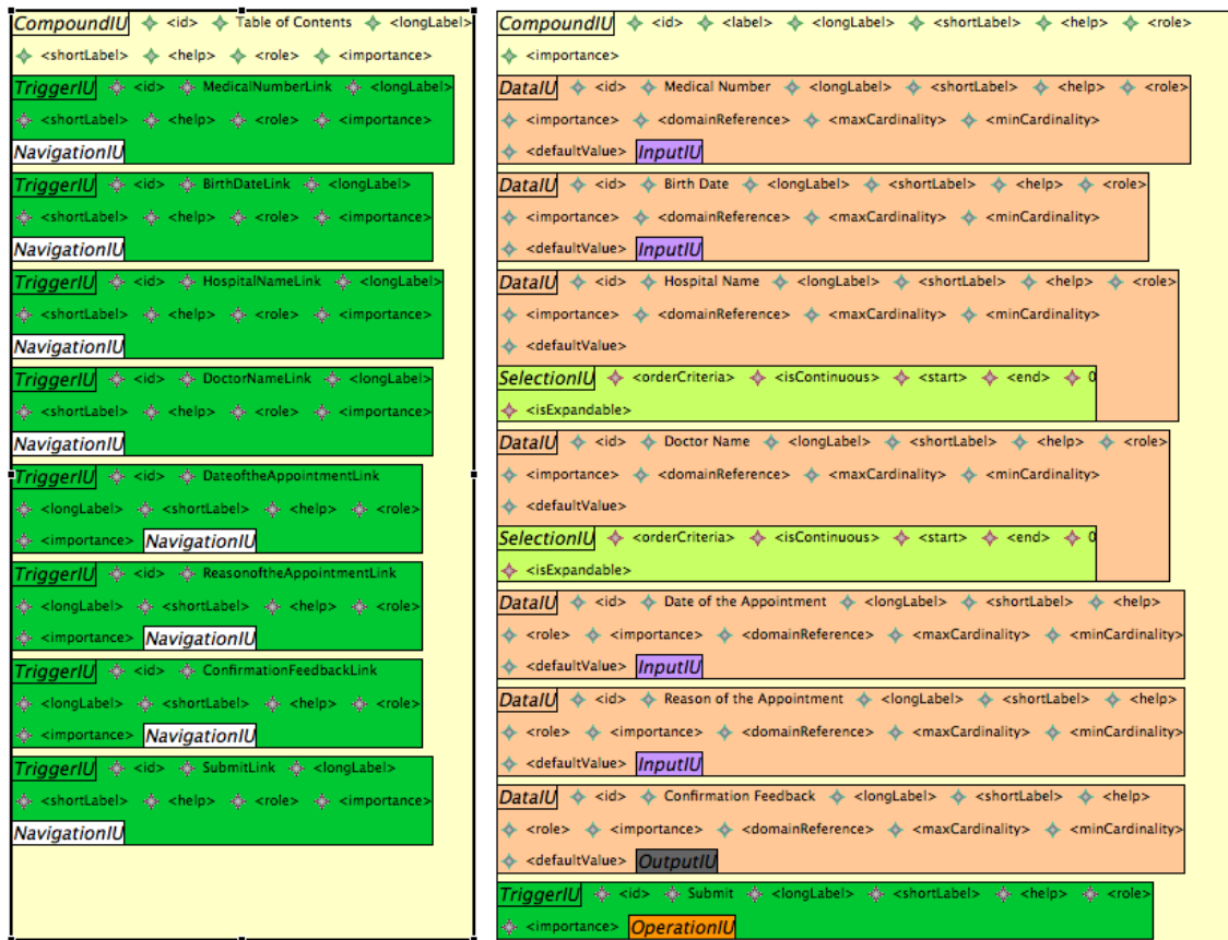
Fig. 10 Tailored abstract user interface for appointments with the doctor. This abstract user interface represents the original application with a table of content added. The yellow rectangle on the left area of the figure represents the table of content inserted after applying the adaptation rules selected, whereas the yellow rectangle on the right area of the figure represents the elements of the original application. The table of content includes a container including a link targeting to each interaction element of the elements of the right area. For instance, on the left area the first navigationUI element is a link identified as MedicalNumberLink . This link targets to the first element on the right area corresponding to an element of type InputUI identified as MedicalNumber .
