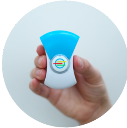
Figure 3.25: A FogSense Wi-Fi sensor used in the measurement campaign.
