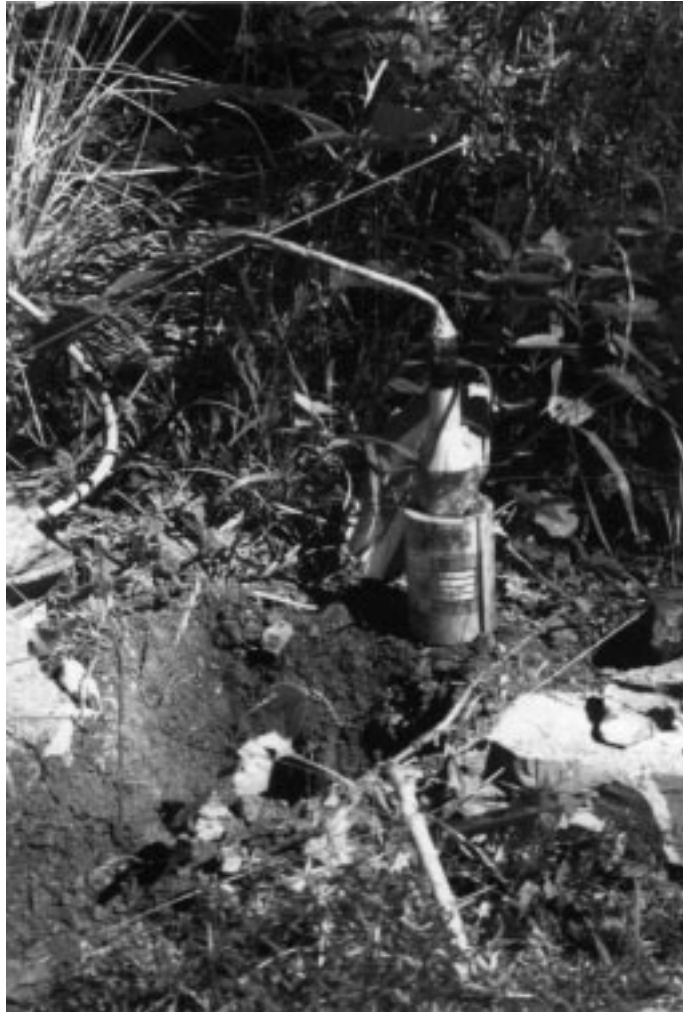
Figure 4. The detectors were placed on the ground in an upright position within a hole about 30 cm deep, subsequently refilled and compacted.
