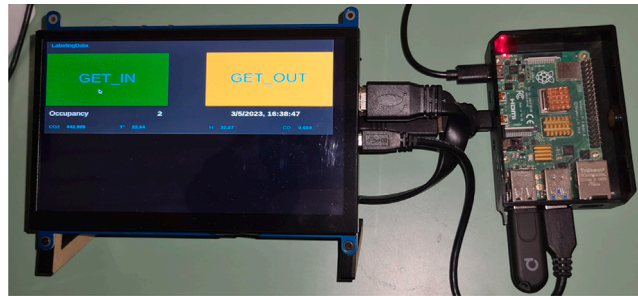
Fig. 4. The touchscreen connected to the EDGE 1 Raspberry Pi.
