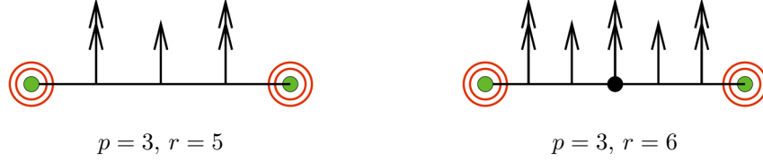
Fig. 1. Triharmonic problem: edge degrees of freedom of the Virtual Element space V_{h,r}(K) . Here, p is the order of the partial differential operator and p = 3 corresponds to the triharmonic case; r = 5, 6 are the integer parameters that specify the maximum degree of the polynomial subspace \mathbb{P}_r(K) of the VEM space V_{h,r}(K) . The (green) dots at the vertices represent the vertex values and each (red) vertex circle represents an order of derivation. The (black) dot on the edge represents the moment of v_h|_e ; the arrows represent the moments of \partial_n v_h|_e ; the double arrows represent the moments of \partial_{nn} v_h|_e .
