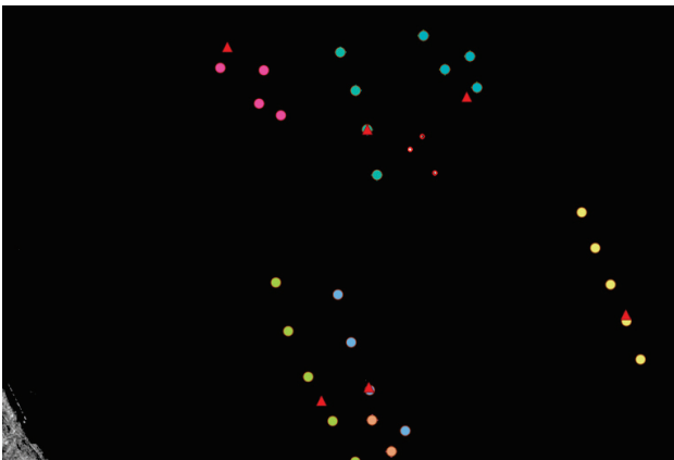
Fig. 6. AIS-SAR matching Case #1 and close up view with SAR targets classified as gas platforms (red circles) and vessels (red triangles). AIS pings are categorized by MMSI.
