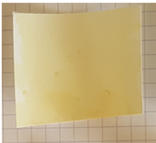
Figure 2. Example of a TFC membrane prepared by coating the Sulzer-PAN support (ca. 5 cm \times 5 cm) with a blend of PIM-EA(Me 2 )-TB and Matrimid ® 5218 at 2 wt.% polymer solution.
