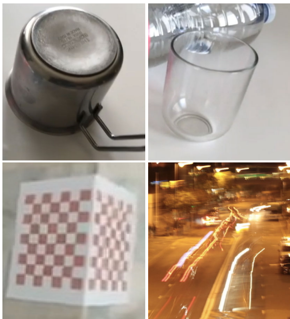
FIGURE 1. Examples of difficult cases for standard SfM pipelines such as reflective, transparent, compressed, and motion-blurred images. Keypoint detection and matching algorithms struggle in such cases, and this results in low-quality 3D models with automatic SfM tools.
