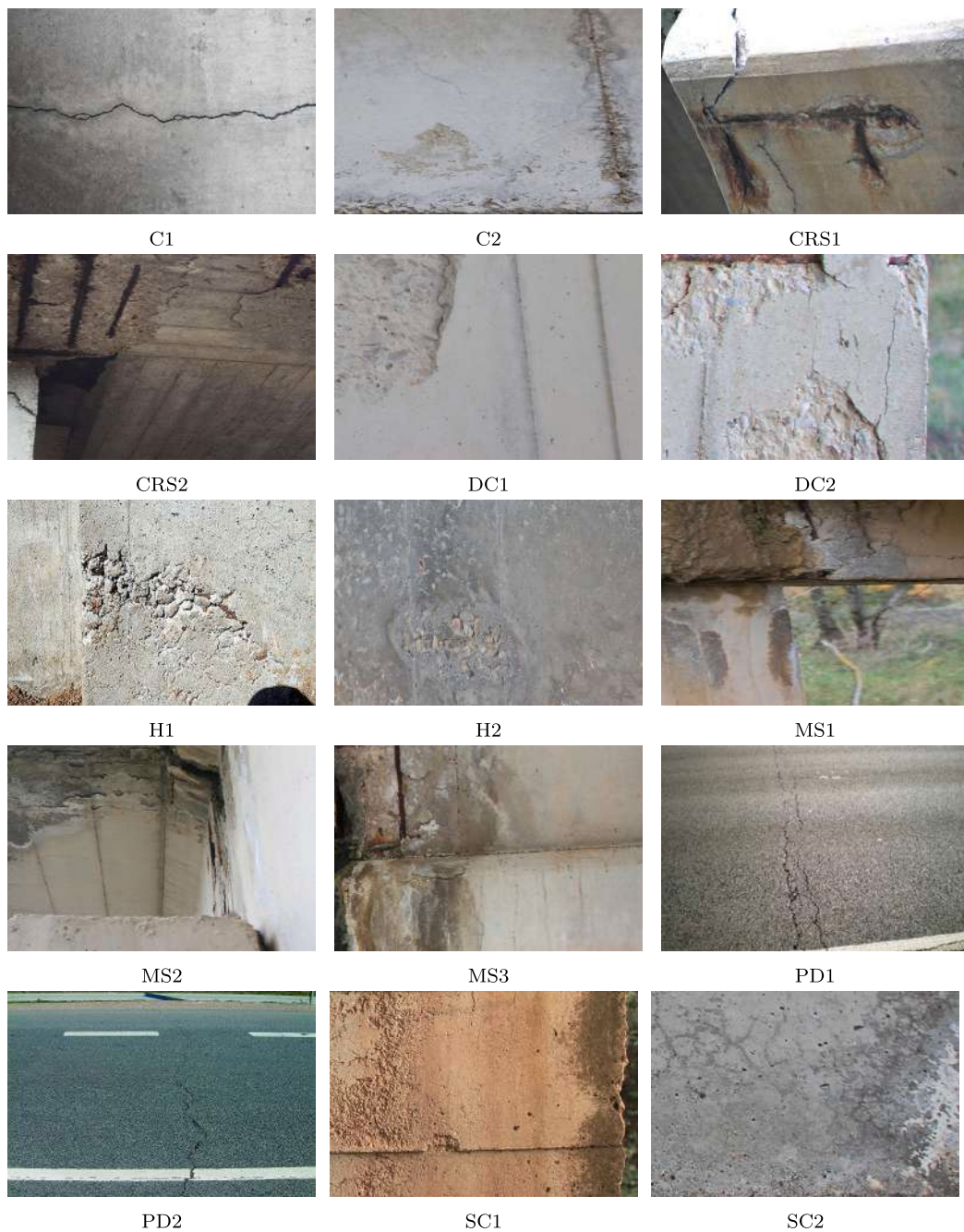
Fig. 4. Images used for the experimental evaluation. Each image characterizes a specific defect, as reported in Table 1; the defect notation, along with a progressive identifier, is used to identify each image univocally.
