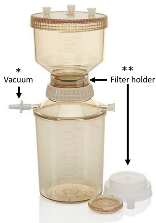
Figure 2. Nalgene™ reusable unit for 250 mL water filtration. Details of vacuum nozzle (*) and filter holder (**).
