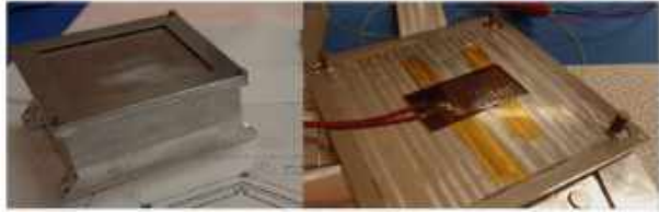
Fig. 21 DISC Unit. Left: assembled DISC breadboard. Right: Sensing plate with glued PZTs at 3 corners
