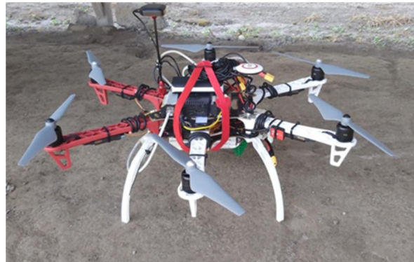
Figure 2. Picture of UAV GPR System 8, Courtesy of Department of Industrial Engineering (DII) of University of Naples, “Federico II”.
