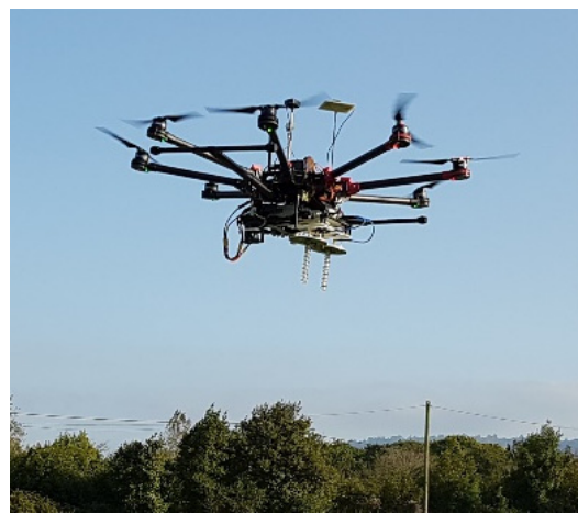
Figure 1. Picture of UAV-GPR System 6. Courtesy of University of Oviedo, Gijón, Spain.
