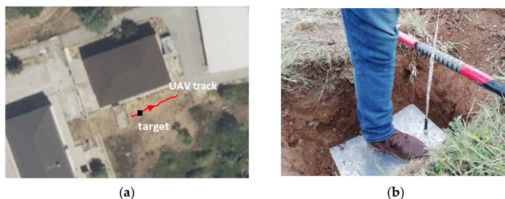
Figure 14. Experimental test site: (a) aerial view of the area with UAV flight trajectory (red line) and target (black rectangle) superimposed; (b) photo of the buried metal plate.
