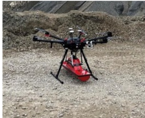
Figure 5. Picture of UAV GPR System 12. Courtesy of Dyrecta Lab., Conversano, Italy.
