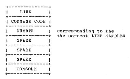
NUMBER will be used by INTERNET as offset in its line-handler table (NTRAVEC) to select the correct line-handler routine address (see STELLA/CNUCE/83/09).
