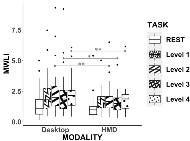
Figure 5. Objective MWL assessment by EEG. The figure shows the boxplots of the mental workload index (MWLI) derived from EEG signals in desktop and HMD conditions. MWLI, in the case of Desktop, had median values of 1.12 at rest, 1.80 in level 1, 2.01 in level 2, 1.87 in level 3 and 2.16 in level 4. Considering HMD, MWLI showed median values of 0.978 at rest, 1.79 at level 1, 1.67 at level 2, 1.51 at level 3 and 1.87 at level 4. The MWLI was significantly lower in HMD than in desktop condition in levels 2, 3 and 4.
