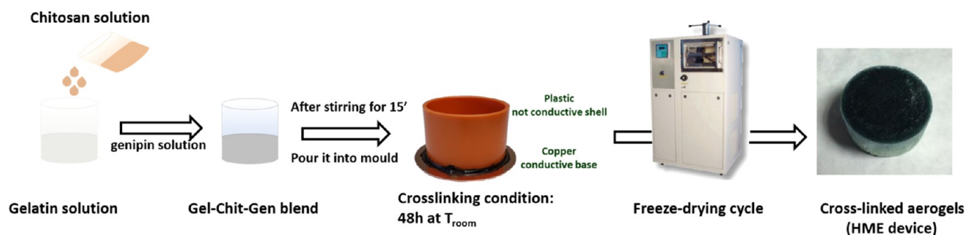
Figure 1. Synthesis and forming process steps to develop the Gel–Chit–Gen aerogel as an HME filter device.
