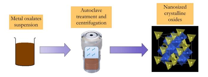
Fig. 1 Combination of coprecipitation of oxalates and hydrothermal treatment
