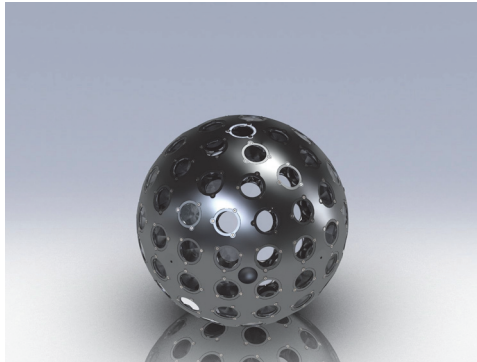
Fig. 3. LARASE rendering of the LARES satellite. LARES is made of a unique piece of tungsten (THA-18N, composition 95% of W and 5% of Cu and Ni) and its surface is covered with 92 CCRs for SLR tracking. The satellite radius is 18.2 cm and its mass is about 386.8 kg. The CCRs mounting system is quite similar to that of the two LAGEOS. The satellite orbit is almost circular with a semi-major axis of about 7820 km (corresponding to an orbital period of about 6883 s). LARES has been launched with the qualification flight of the new European launcher VEGA. We refer to 9,10 for further details.
