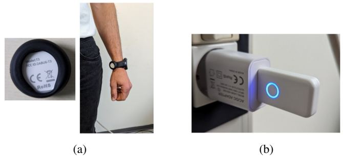
Fig. 1: (a) Bluetooth tag on the left side encapsulated within a silicon box and (b) Bluetooth gateway plugged to an USB adapter.
