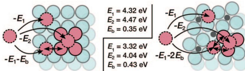
Fig. 3. – Sketch of three different steps possibly occurring in the process of Co aggregation on Ni(100) (left) and Ni 2 C (right): 1) adsorption of an individual Co adatom (energy gain: -E_1 ); 2) addition of a Co adatom to the first layer of an existing island (with a further energy gain of -E_b for each Co-Co bond in the first layer); 3) addition of a Co adatom in the second layer (with a further energy gain of -E_2 for each Co-Co bond between the two layers).
