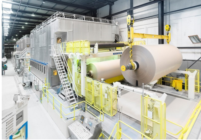
Figure 1: A paper machine with jumbo rolls in the foreground (from VOITH)
