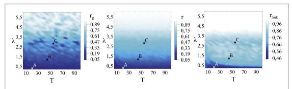
**Figure 2.** The global order parameter (a), the layer order parameter (b) and the local order parameter (c) as functions of the coupling strength  $\lambda$  and the adaptation time T. Points labeled with A, B and C correspond to three particular system's configurations that will receive specific attention in our paper.
