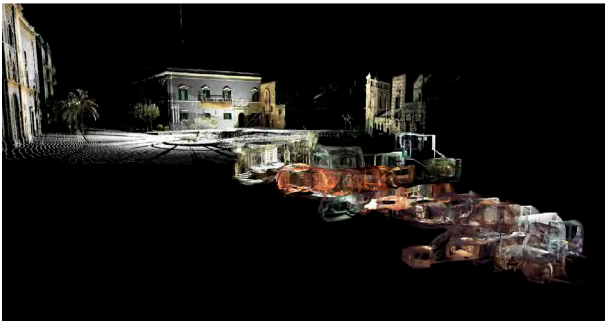
Figure 10. The laser scanner survey of the hypogea area in the city of Matera—Piazza “Vittorio Veneto”—Image and laser scanner survey worked out by Matheca s.r.l. in Matera.
