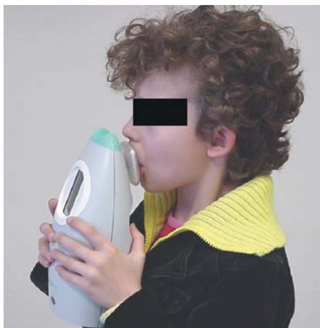
Figure 1. Measurement of F_{\text{ENO}} in a child using a hand-held device with an electrochemical sensor. Maintaining a low, constant expiratory flow is facilitated by optical, auditory and visual feedback signals. The result is immediately available.
