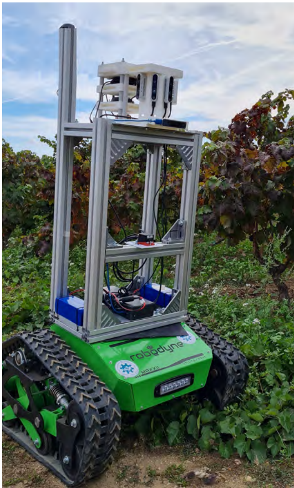
Figure 6: Robotic platform used for in-field testing equipped with the multi-sensor box.
