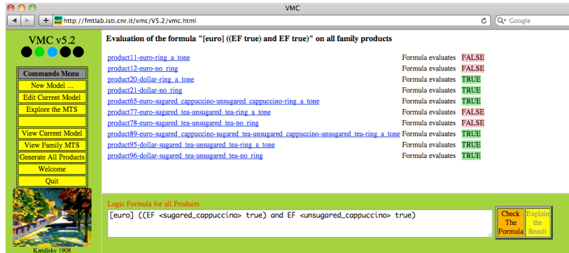
Fig. 4. All valid products/LTSs of the family/MTS of Fig. 3 as generated by VMC and the result of model checking a variant of Property 2 over all valid coffee machines
