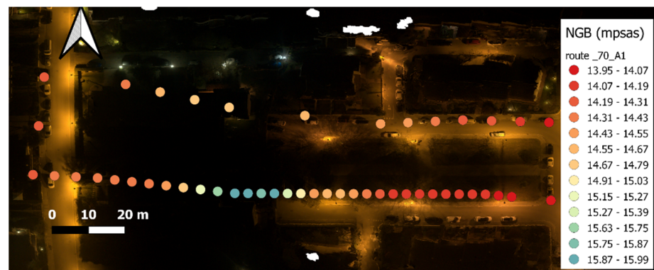
Figure 9. Georeferenced night ground brightness (NGB) measured in magnitude/arcsec 2 (mpsas) recorded by the UAV along the route at 70 m height on 3 April 2021 displayed upon the georeferenced night images taken by the digital camera during the same flight. Colors indicate NGB in mpsas.
