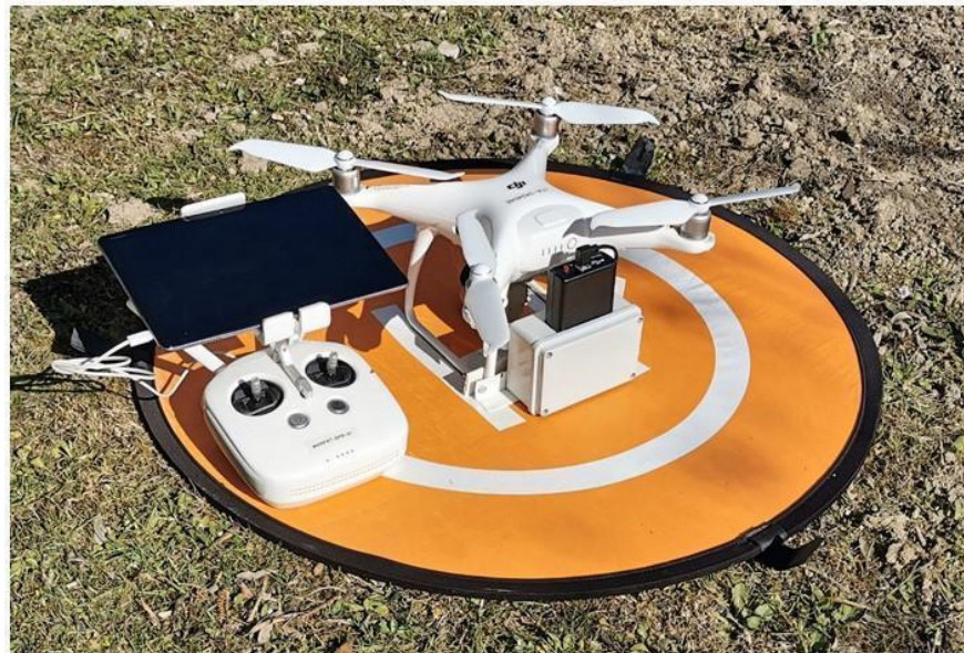
Figure 2. Sky quality meter (SQM) mounted on the unmanned aerial vehicle (UAV).
