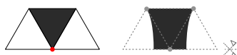
Fig. 12. Filleting interface vertices that lie on the polygon edge. Gray dots indicate Bézier control points.
