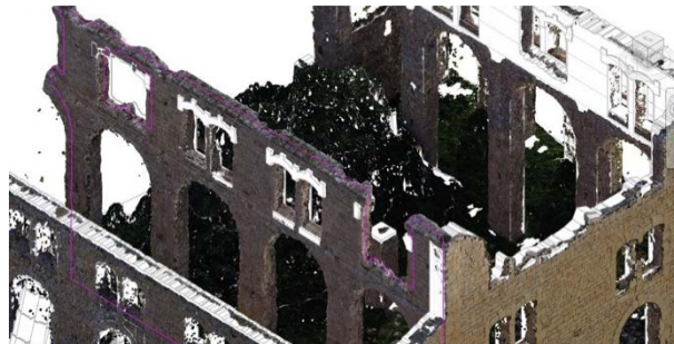
Fig. 2. Visualization of the BIM modelling of the walls of the Fornace Penna over its point cloud.
