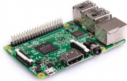
Fig. 1: Raspberry PI 3 model B: a credit-card-sized computer that features an ARM CPU (quad core 1.2GHz Broadcom BCM2837 64bit), a Wi-Fi chipset (Broadcom BCM43438), 1GB RAM.
